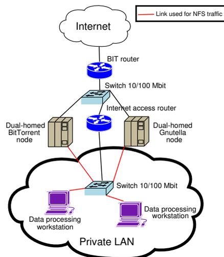
Figure 5: Distributed measurement setup
